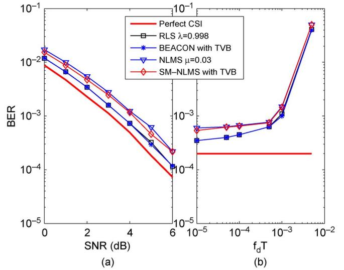
Fig. 15. (a) BER performance versus SNR for quasi-static fading channel and (b) BER performance versus  $f_d T$  (SNR = 5 dB) for Rayleigh fading channels.  $n_p = 1000$ ,  $n_t = 100$ , and  $n_d = 900$ .
