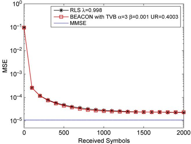
Fig. 9. MSE performance of the BEACON channel estimation with a TVB for quasi-static fading channel.  $n_p = 2000$ ,  $n_t = 100$ , and  $n_d = 1900$ .
