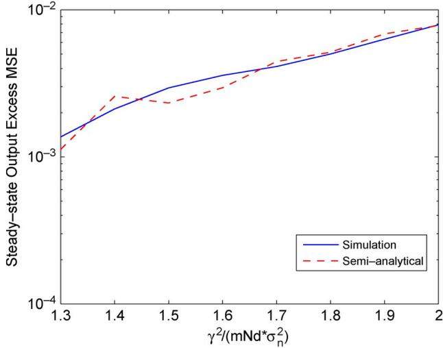
Fig. 18. Steady-state excess MSE analysis for the BEACON channel estimation.
