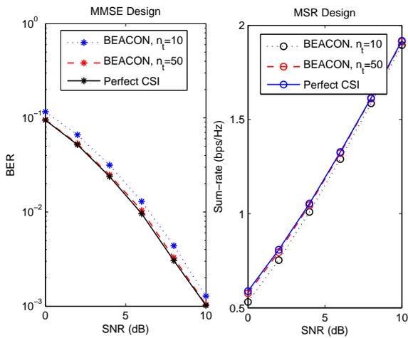
Fig. 11. (a) BER performance versus SNR of our proposed MMSE design (b) Sum-rate performance versus SNR of our proposed MSR design with a global power constraint when employing the BEACON channel estimation, compared to the performance of perfect CSI
