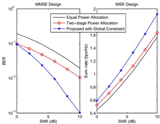
Fig. 9. (a) BER performance versus SNR of our proposed MMSE design (b) Sum-rate performance versus SNR of our proposed MSR design with a global power constraint and compare with the two-stage power allocation and equal power allocation schemes.
