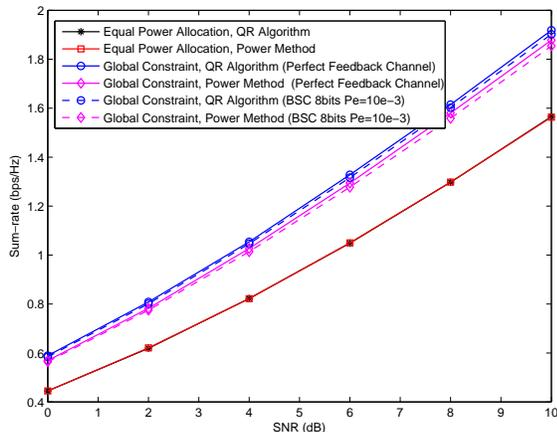
Fig. 5. Sum-rate performance versus SNR of our proposed joint MSR design of the receiver and power allocation strategies with a global constraint, compared to the equal power allocation method.
