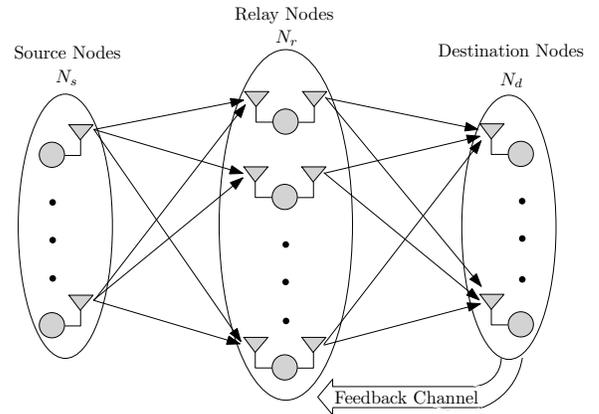
Fig. 1. A two-hop cooperative WSN with  $N_s$  source nodes,  $N_d$  destination nodes and  $N_r$  relay nodes.
