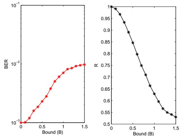
Fig. 7. (a) BER performance versus the bound and (b)  $R$  versus the bound of the MMSE design with a neighbour-based power constraint.
