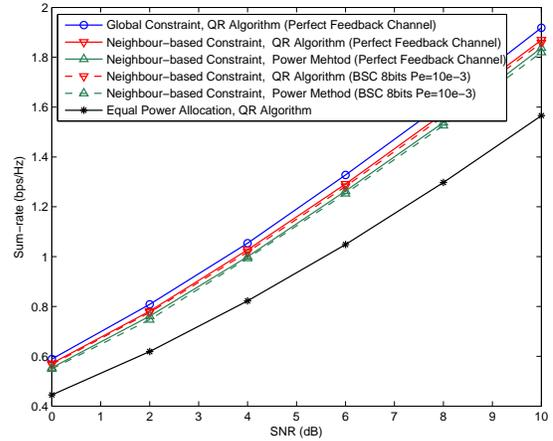
Fig. 6. Sum-rate performance versus SNR of our proposed joint MSR design of the receiver and power allocation strategies with a neighbour-based constraint, compared to the equal power allocation method.
