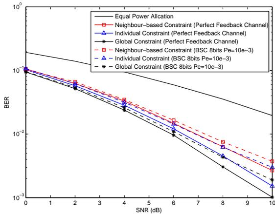
Fig. 4. BER performance versus SNR of our proposed joint MMSE design of the receiver and power allocation strategies, compared to the equal power allocation method.
