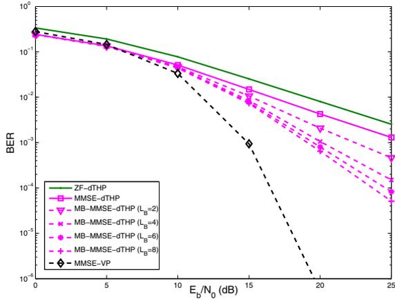
Fig. 6: BER performance of dTHP,  $(2, 2, 2, 2) \times 8$  MIMO, 16-QAM.
